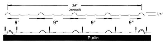
PortaGrace Mfg. recommends the use of painted or galvanized screws as a fastening method for our metal panels. Screws should have a driller tip with a flat rubber washer being careful to apply sufficient torque to seat the washer – do not overdrive the fastener.
